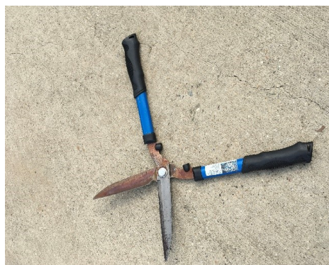
Figure A: Garden Shears lost for several years. Shiny blade rubbed with lemon half for 15 seconds then rinsed, wiped dry, and lightly oiled. I plan to finish this project next week by taking a part and thoroughly cleaning, removing all rust, drying, oiling exposed metal, sharpening cutting edges, candle wax on mating surface, and reassembly.
