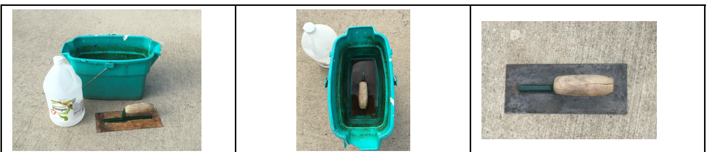
Figure 4: This trowel was left in my garden tool bucket after using last season and surface rust formed on it. I placed it in a paint pail and covered the rusted area with vinegar. About 10 hours later, the rust was replaced with a blackened coating which I wanted. I just rinsed, wiped dry and oiled. For a thicker and richer black coating leave in the vinegar longer, then rinse, wipe dry, and polish with fine steel wool before oiling. Caution: Wear surgical gloves when cleaning black residue off tool as the residue stains.
